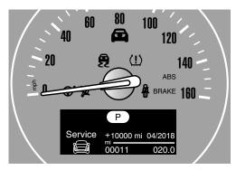
The remaining driving distance and the date of the next scheduled service are briefly displayed in the speedometer immediately after you start the engine or switch on the ignition.
