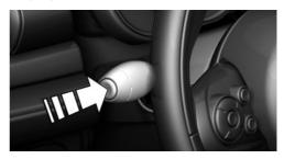
Press and hold button on blinker lever.
