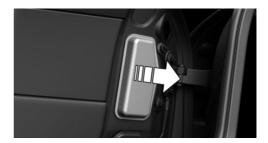
Press the latches together upward, arrow 1, and remove the bulb holder. Loosen the plug connector, arrow 2, on the bulb holder.
