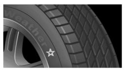
For each tire size, the manufacturer of the vehicle recommends certain tire brands. These can be identified by a star on the tire sidewall.
