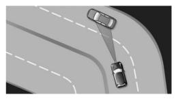
When you approach a curve the system may briefly report vehicles in the next lane due to the bend of the curve. If the system decelerates you may compensate it by briefly accelerating. After releasing the gas pedal the system is reactivated and controls speed independently.
