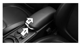
Lower storage compartment: press button, arrow 1, and fold the center armrest up, arrow 2.
