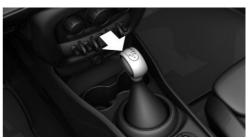
Press unlock button on the front of the selector lever, arrow.
