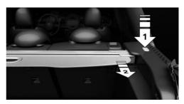
Press the release button, arrow 1, and pull the cargo cover out towards the rear, arrow 2.
