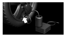
With the compressor switched off, insert the plug into the power socket inside the vehicle.
