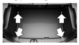
With storage package: to secure the cargo there are four lashing eyes in the cargo area.
