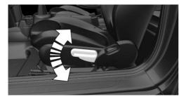
Pull the lever up or press it down as often as needed to reach the desired height.
