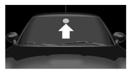
The camera is installed near the interior mirror. Keep the windshield in the area behind the interior mirror clean and clear.
