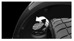
Pull bulb holder out of the bulb housing; if needed, loosen it with small tilting movements if possible.
