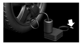
With operating readiness switched on or the engine running, switch on the compressor.
