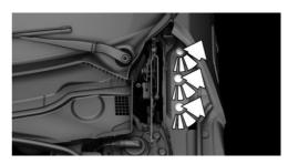
Turn the bulb holder counterclockwise and remove.
