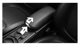
Upper storage compartment: press button, arrow 1, and fold the center armrest up, arrow 2.
