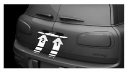
Unlock the vehicle and use the button in the handle to completely open first the right side, arrow 1, and after that the left side of the split doors, arrow 2.
