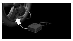
Insert the connector into a power socket inside the vehicle.
