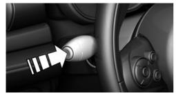
Press button on the turn signal lever several times if needed.
