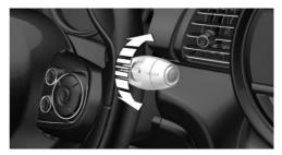
Turn the thumbwheel to adjust the frequency or sensitivity of the rain sensor.
