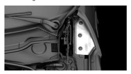
Loosen nuts of the cover by hand and remove the cover.
