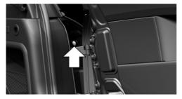
3. Briefly press the rear edge of the fuel filler flap. Fuel filler flap is opened.
