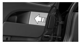
Press the latches together in the direction of the arrow, arrow 1, and remove the bulb holder.
