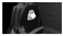
Turn the bulb holder for the reversing light, arrow, counterclockwise and remove it.
