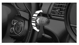
Turn the thumbwheel on the wiper lever.
