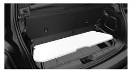
Grasp the cargo floor panel in the rear and fold slightly upward. Next, pull it backward from the supports.
