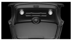
Recessed grips on the interior trim of the tailgate can be used to conveniently pull down the tailgate.
