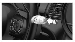
Press the button on the wiper lever.
