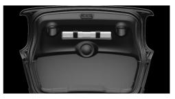
The warning triangle is located in the tailgate. To remove, loosen the brackets.
