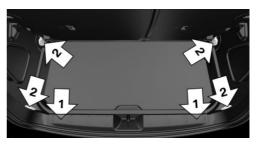
Without storage compartment package: to secure the cargo there are two lashing eyes, arrow 1, in the cargo area.
