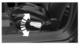
Pull the lever up or press it down as often as needed to reach the desired height.
