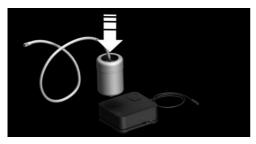
4. Screw the filling hose of the sealant container onto the tire valve of the nonworking wheel.
