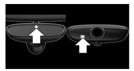
Photocells are used for control:
