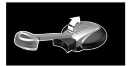
3. Slide the integrated key in the cover of the battery compartment and raise the cover.
