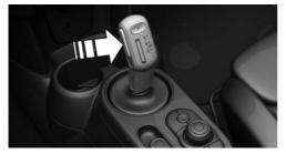
2. With the driver's safety belt fastened, briefly push the selector lever in the desired direction, past a resistance point, if needed. The selector lever automatically returns to the center position when released.
