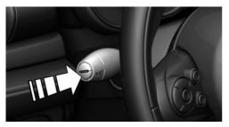
Position of switch: ∰C Press the button on the turn signal lever.
