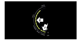
The energy recovery occurs during coasting and braking and is displayed in the performance display by the accelerator pedal indicator. The accelerator pedal indicator is within the CHARGE range.
