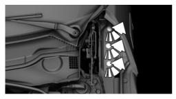
3. Turn the bulb socket counterclockwise and remove.
