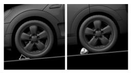
If you need to change a wheel on a slight downhill grade, place chocks and other suitable objects, for instance a rock, under the wheels of both the front and rear axles against the rolling direction.
