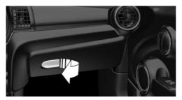
Pull the handle. The light in the glove compartment switches on.
