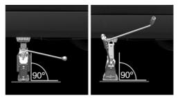
7. Crank the vehicle up, until the vehicle jack is with the entire surface on the
