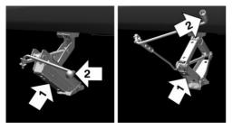
2. Insert the vehicle jack into the rectangular recess of the jacking point closest to the wheel to be changed.
