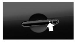
Press and hold down the button on the driver's or front passenger's outer door handle.
