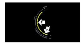
Pointer in the CHARGE range, arrow 1: display for energy recovery by coasting or when decelerating:
