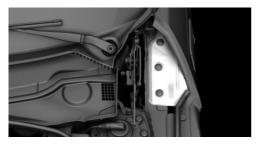
2. Loosen the nuts of the cover by hand or with the onboard vehicle tool kit, refer to page 250, and remove the cover.
