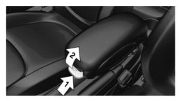
Press button, arrow 1, and swing center armrest upward or downward into the desired height, arrow 2.
