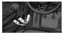
After the lever is released, pull the lever again, arrow 2. Hood can be opened.
