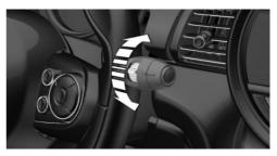
Turn the thumbwheel on the wiper lever.
