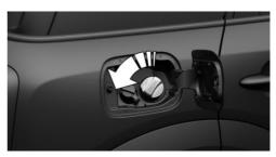
3. Place the fuel cap in the bracket attached to the fuel filler flap.
