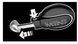
Press the button, arrow 1, and pull out the integrated key, arrow 2.
