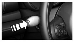
Press and hold button on signal lever.
