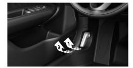
2. After the lever is released, pull the lever again, arrow 2. Hood can be opened.
