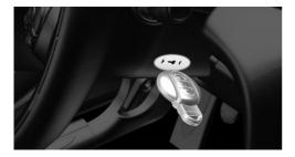
It is not possible to start the engine if the remote control has not been detected.
