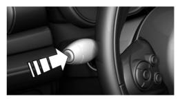
Press button on the turn signal lever several times, if needed.
