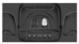
The indicator light for the front-seat passenger airbags indicates the operating state of the front-seat passenger airbags.
