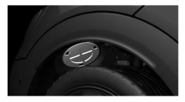
3. Unscrew the inner cover counterclockwise, and remove it.
