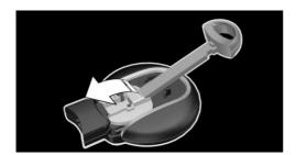
4. Push battery in the direction of the arrow using a pointed object and lift it 011f.
