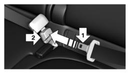
Guide the safety belt to the mount in the roofliner.
