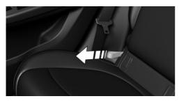
Pull the strap and apply your weight to the backrest or lift it off, as necessary.
