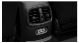
One USB dual charge socket is located in the rear center console.
