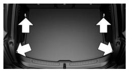
With storage compartment package: to secure the cargo there are four lashing eyes in the cargo area.
