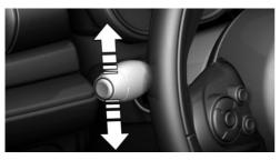
With radio-ready state switched off, press the lever either up or down past the resistance point for approx. 2 seconds.
