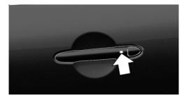
On the driver's or front passenger's outer door handle, press the button.
