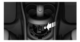
4. Press the button on the front of the selector lever and move the selector lever back slightly.
