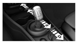
The selector lever positions P, R, N, and D are selected by tapping the selector lever
