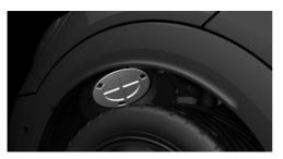
3. Unscrew the inner cover counterclockwise, and remove it.
