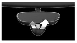
To reduce the blinding effect of the interior mirror, flip the lever forward.
