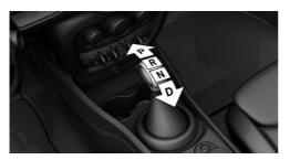
The selector lever positions P, R, N, and D are selected by moving the selector lever into the respective selector lever position. The selector lever engages in the selector lever positions.
