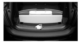
3. Fold the rear part of the cargo area floor downward and place the MINI Picnic Bench over the loading lip of the cargo area. Place a protective cloth over the bumper.
