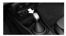
2. Move the selector lever into the desired position.
