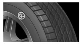
The tires are marked on the tire sidewall with RSC Run-flat System Component.
