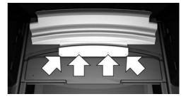
Fold down the MINI Picnic Bench toward the rear. The MINI Picnic Bench is fastened with magnets.
