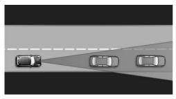
The detection capacity of the system and the automatic braking capacity are limited. Two-wheeled vehicles for instance might not be detected.
