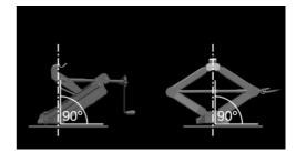
6. Make sure that the vehicle jack foot stands vertically and perpendicularly beneath the jacking point after extending the vehicle jack.
