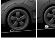
If you need to change a wheel on a slight downhill grade, place chocks and other suitable objects, for instance a rock, under the wheels of both the front and rear axles against the rolling direction.
