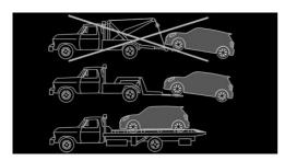
Your vehicle should be transported with a tow truck with a so-called lift bar or on a flat bed.
