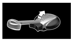
3. Slide the integrated key in the cover of the battery compartment and raise the cover.
