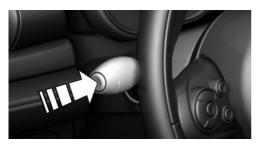
Press and hold button on signal lever. Information is displayed in the Info Display of the instrument cluster.
