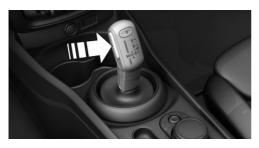
With the driver's safety belt fastened, briefly push the selector lever in the desired direction, past a resistance point, if needed. The selector lever automatically returns to the center position when released.
