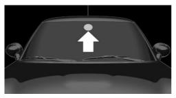
The camera is installed near the interior mirror.
