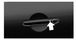
Press and hold down the button on the driver's or front passenger's outer door handle.
