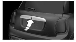
Without Comfort Access: unlock vehicle. With Comfort Access: unlock the vehicle or have the remote control with you. Press button next on tailgate.
