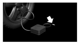
5. With the ignition switched on or the engine running, switch on the compressor. If a tire inflation pressure of at least 2 bar cannot be reached, contact your dealer's service center or another qualified service center or repair shop.
