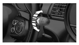
Turn the thumbwheel on the wiper lever.
