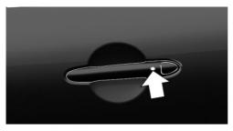
On the driver's or front passenger's door handle, press the button.
