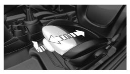
Pull the lever at the front of the seat and adjust the thigh support.
