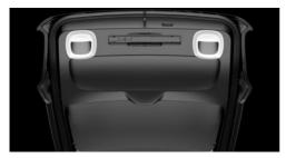
Recessed grips on the interior trim of the tailgate can be used to conveniently pull down the tailgate.
