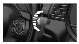
Turn the thumbwheel on the wiper lever.
