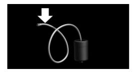
3. Slide the sealant container into the holder on the compressor housing, ensuring that it engages audibly.
