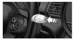
Press the button on the wiper lever.
