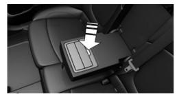
Pull the center armrest forward at the strap. To open: press the button.
