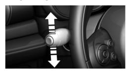
Press the lever past the resistance point. Canada: the lever returns into its starting position after actuation. To switch off manually, slightly tap the lever to the resistance point.
