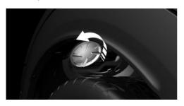
4. Turn the bulb holder counterclockwise, arrow 1, and remove, arrow 2.
