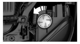
3. Tilt the bulb holder up, arrow 1, and pull it out of the headlight toward the rear, arrow 2.
