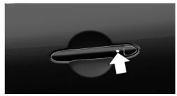
On the driver's or front passenger's outer door handle, press the button.
