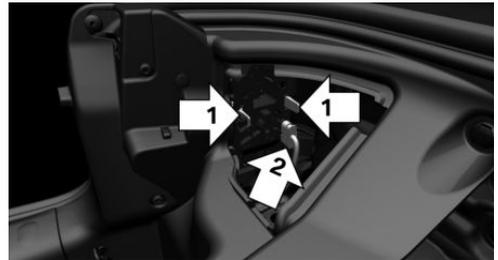
4. Remove the bulb holder from the opening.
