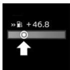
The bar display below the tachometer is filled in green and the mark appears at the zero point. The tachometer shows the idle speed.
