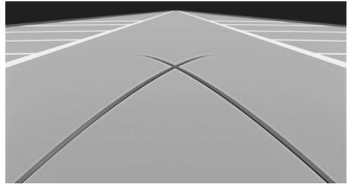
Turning radius lines can be superimposed on the image of the rearview camera.
