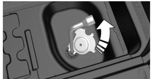
5. Lower the emergency wheel with the wheel wrench.
