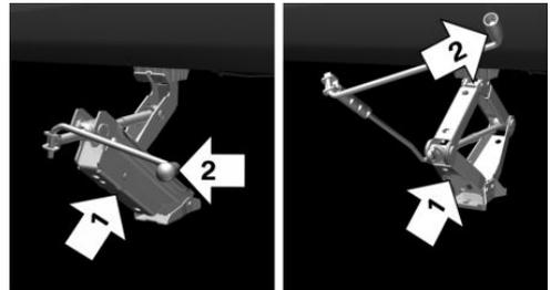
2. Insert the vehicle jack into the rectangular recess of the jacking point closest to the wheel to be changed.
