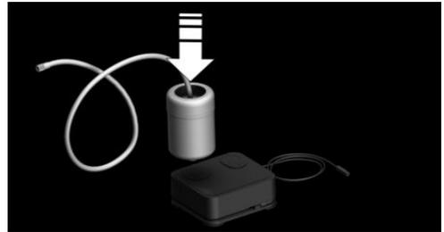
4. Screw the filling hose of the sealant container onto the tire valve of the non-working wheel.
