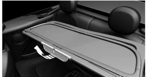
4. Press the wind deflector inwardly and up, arrow 1, to the extent that the wind deflector can be positioned in front of the fixing points on the installation side. Release the handle.
