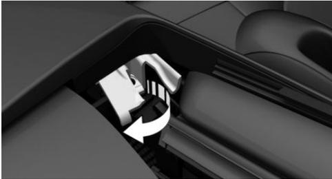
5. Loosen and remove the two screws on both sides of the vehicle using the hexagon wrench.
