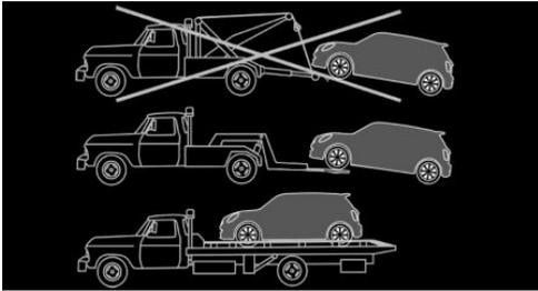
Have your vehicle transported with a tow truck with a so-called lift bar or on a flat bed.
