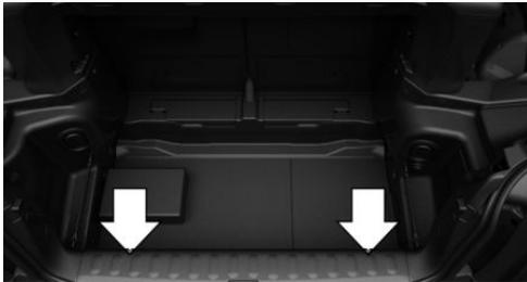
To secure the cargo there are two lashing eyes in the cargo area.
