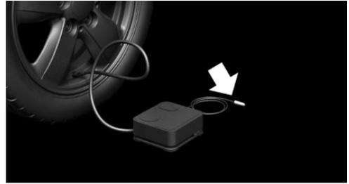
4. Correct the tire inflation pressure to at least 2.0 bar.
