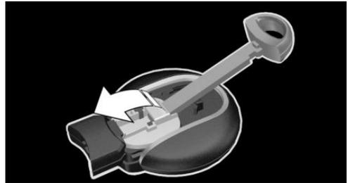
4. Push battery in the direction of the arrow using a pointed object and lift it out.
