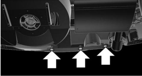
2. Push the heat shield forward and the bumper back in order to be able to reach the fog light.
