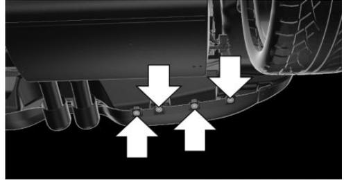
2. Push the heat shield forward and the bumper back in order to be able to reach the fog light.
