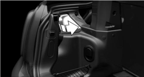
3. Turn the bulb holder for the reversing light, arrow, counterclockwise and remove it.
