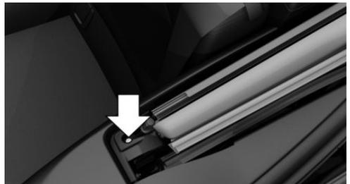
2. On the left side of the vehicle only: raise the cover and pull the sensor outward and off.
