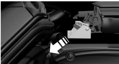
6. Insert the pins on the side frames into the receptacles on the windshield frame.
