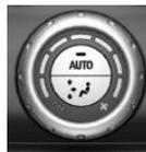
Turn the ring to set the desired air flow.
