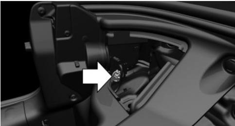
4. Remove the bulb holder from the opening.
