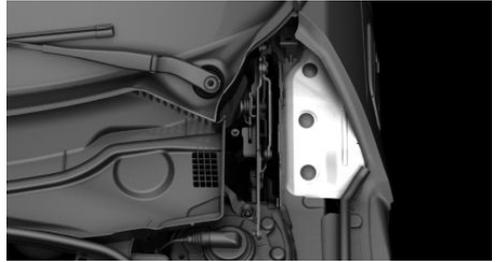
2. Loosen nuts of the cover by hand and remove the cover.
