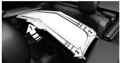
5. Press the wind deflector downward in the middle, until the handle engages, arrows 1.
