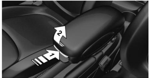
Press button, arrow 1, and open center armrest upward, arrow 2.
