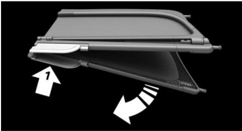
2. Open the rear side window, if necessary. Insert wind deflector from one side of the vehicle with the pins in the corre-
