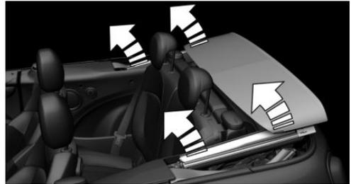
3. In the vehicle, lift the cover in the center of the roof using the screwdriver.
