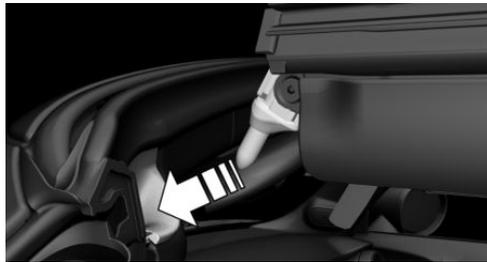
7. Turn the hexagon wrench clockwise to close the side frame lock.
