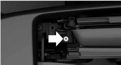
6. Only on the left side of the vehicle: slightly lift the side frame, arrow 1, and pull the sensor with the cable forward out from the guide, arrow 2.
