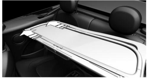
3. To release the lock, fold the handle up and hold it.
