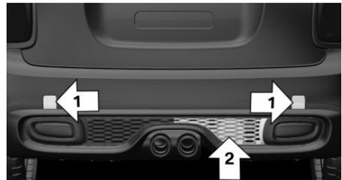
The fixing points, arrow 1, and the socket, arrow 2, are located below the covers in the bumper.
