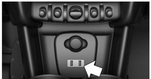
Depending on the vehicle equipment, one or two USB interfaces are located in the front of the center console.
