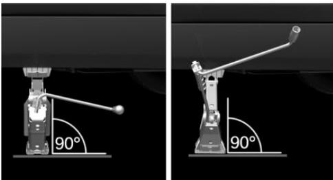
7. Crank up the vehicle jack until the entire surface of the jack is in contact with the ground and the wheel in question is
