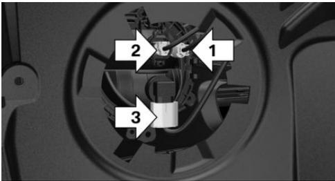
5. Pull the bulb out of the fixture.
