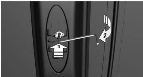
5. Pull of the locking elements from the pins on the left and right side of the side frames, arrow.
