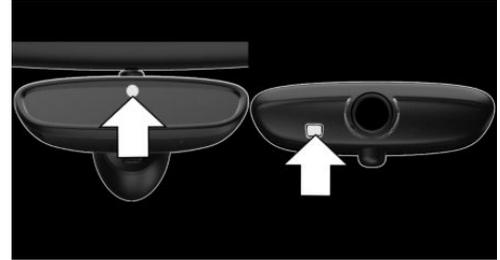
Photocells are used for control:
