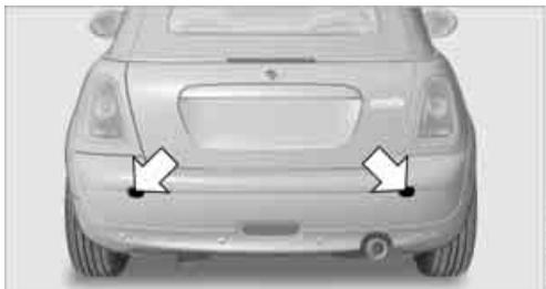
The mounting points are under the protective caps in the bumper. Push out the caps at the respective slots.
