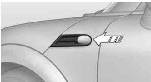
2. Unscrew the bulb holder counterclockwise.
