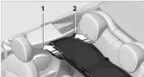
1. Push out retaining pin 2 on one side until it engages.
