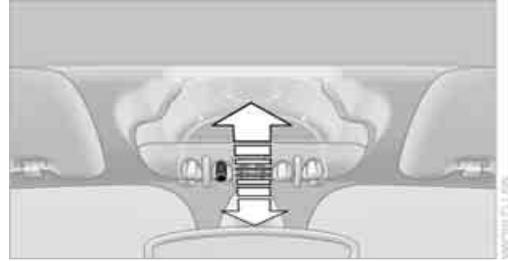
To switch the interior lamps on/off.
