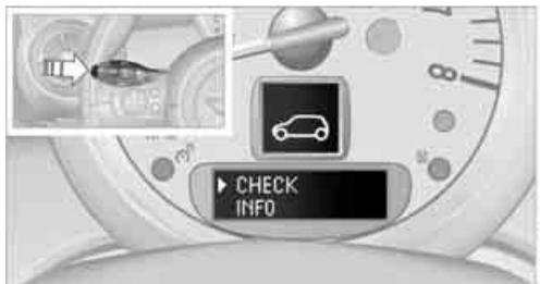
4. Press and hold the button. If there are no Check Control messages, then "CHECK OK" is displayed. If a Check Control message has been stored, the corresponding message is displayed. In addition, the text message appears on the Control Display.
