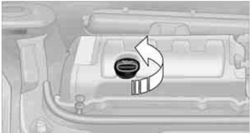
Do not add the maximum quantity of 1 US quart/1 liter of engine oil until the oil level has dropped to just above the lower mark on the dipstick, page 215.
