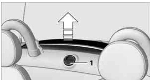
2. Guide the convertible top forward to the windshield frame. Get out of the vehicle if necessary.
