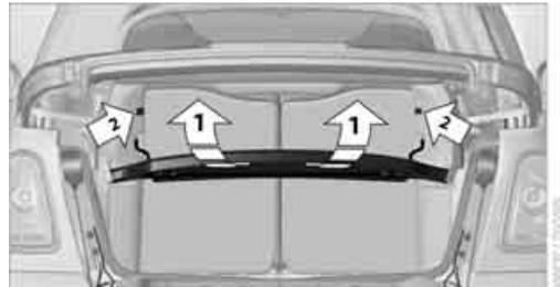
2. Pull luggage compartment roller cover rearward out of the lower brackets and pivot upward, refer to arrows 1,
