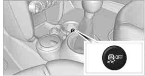
Press the button; the indicator lamp DSC OFF on the speedometer comes on and TRACTION is displayed on the tachometer.
