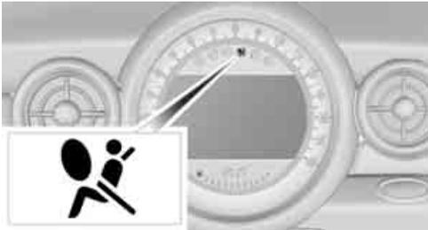
When switching on the ignition, page 54, the warning lamp lights up briefly to indicate that the entire airbag system and the belt tensioners are operational.
