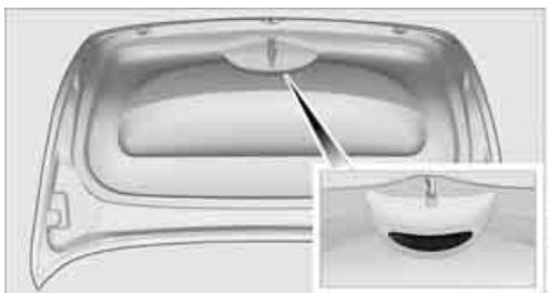
A handle recess on the interior trim panel of the tailgate make it easier to pull it down.
