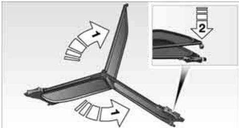
3. Press the locking device together until it engages, refer to arrow 2.
