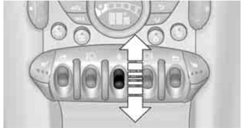
The switch locks or unlocks the doors and tail-gate when the doors are closed, but the anti-theft system is not activated. The fuel filler flap remains unlocked.
