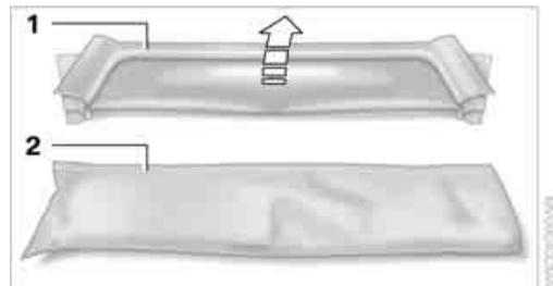
Fold the wind deflector 1 closed and slide it into the storage pouch 2.
