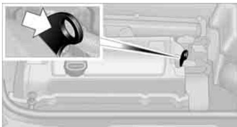
6. Attach the second terminal clamp of the minus/- jumper cable to the negative terminal of the battery or to the engine or body ground of the vehicle to be started.
