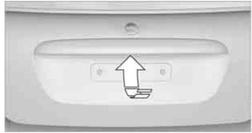
Press the button in the handle, arrow, or the
