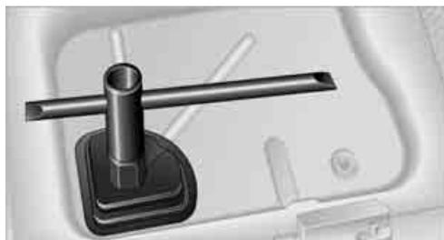
3. Screw the lifting handle from the toolkit onto the thread.
