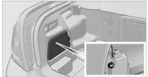
2. Pull on the green knob with the fuel pump symbol. The fuel filler flap is released.
