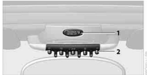
1 Indicator/warning lamp for front passenger airbags 86
