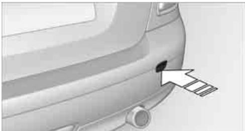
John Cooper Works with aerodynamic bumper: Pull out the bottom of the cover panel of the towing eye in the bumper, arrow.
