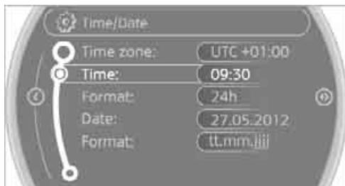
4. Turn the MINI joystick to set the hours and press the MINI joystick.
