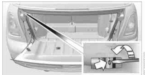
3. Use the screwdriver and turn the gold-colored screw, refer to arrow, one and a half turns in the direction of the arrow.
