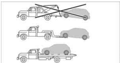
Have the MINI transported by a tow truck with a so-called lift bar or on a flat bed.
