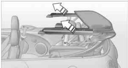
2. Lift out both sides at the same time, and swing the convertible top forward onto the cowl.
