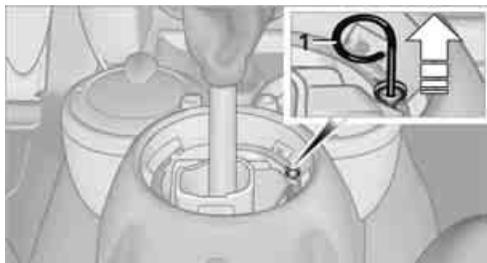
3. Insert extractor hook 1 from the toolkit into the loop on the passenger's side.
