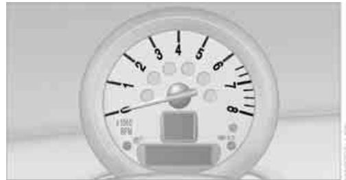
Never operate the engine with the needle in the red overspeed zone of the gauge. In this range, the fuel supply is interrupted to protect the engine.
