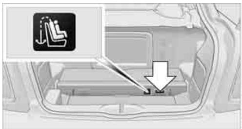
For child restraint systems with tether straps, there is an additional anchor, arrow.
