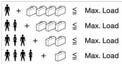
The permissible load is the sum of the occupants' weights and the weight of the cargo. The greater the weight of the occupants, the less cargo/luggage can be transported.
