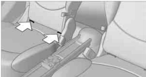
The mounts for the lower LATCH anchors are located at the points indicated by the arrows.
