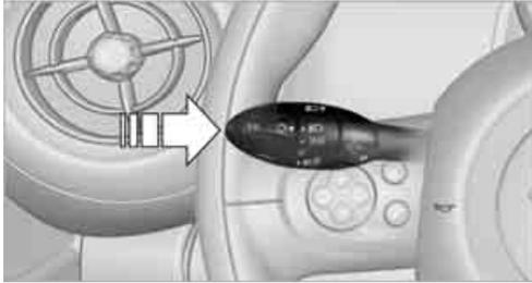
Press the button in the turn signal lever.
