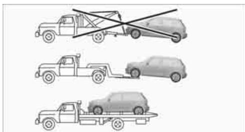
Have the MINI Countryman transported by a tow truck with a so-called lift bar or on a flat bed.
