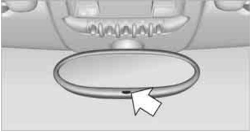
It is controlled by two photosensors:
