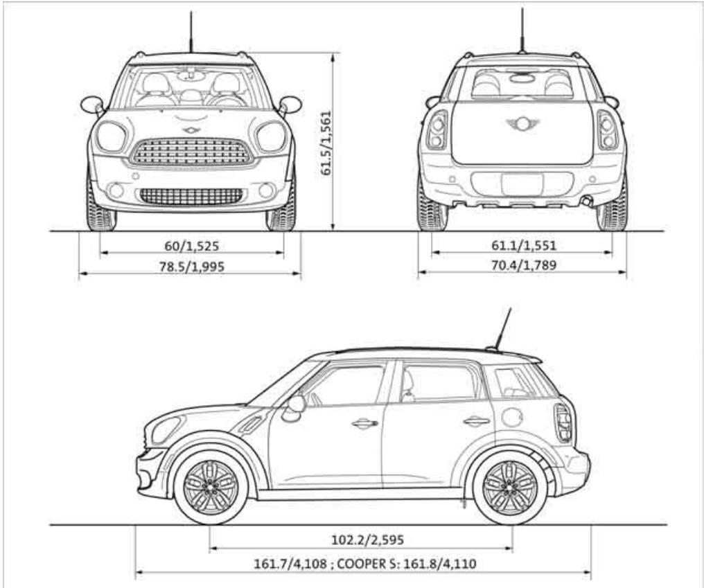
All dimensions in inches/mm. Minimum turning radius dia.: 38.1 ft/11.6 m.
