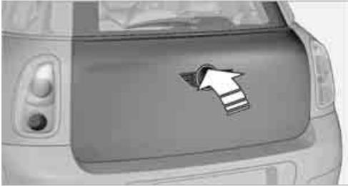
Press the top side of the MINI emblem, arrow, or Press the
