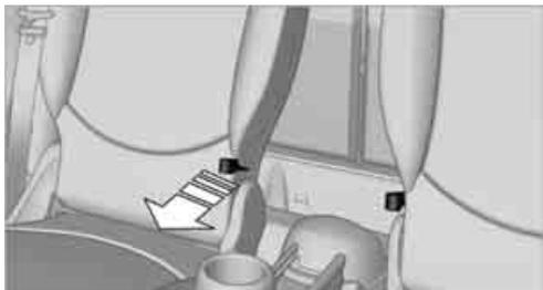
1. Hold on to the backrest near the top, for example on the headrest, and pull on the loop, arrow.
