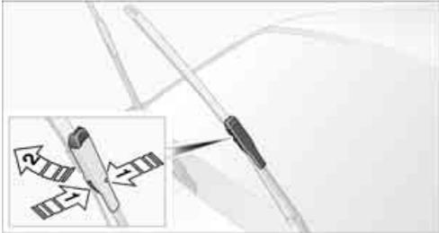
2. Press together the locking spring, arrows 1, and fold out the wiper blade, arrow 2.
