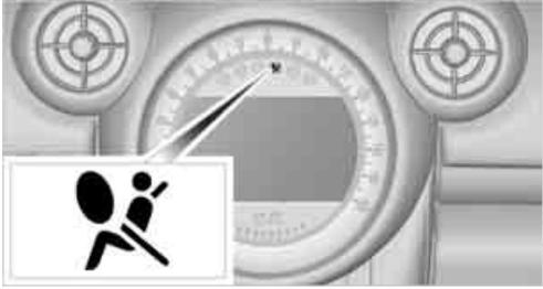
As of radio readiness, page 46, the warning lamp lights up briefly to indicate that the entire airbag system and the belt tensioners are operational.
