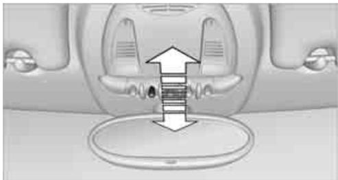
To switch the interior lamps on/off.
