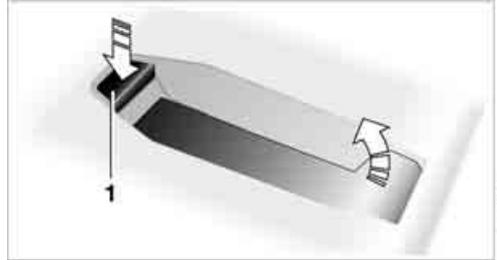
2. Insert the snap-in adapter at the front, arrow 1, and press downward, arrow 2, until it clicks into place.
