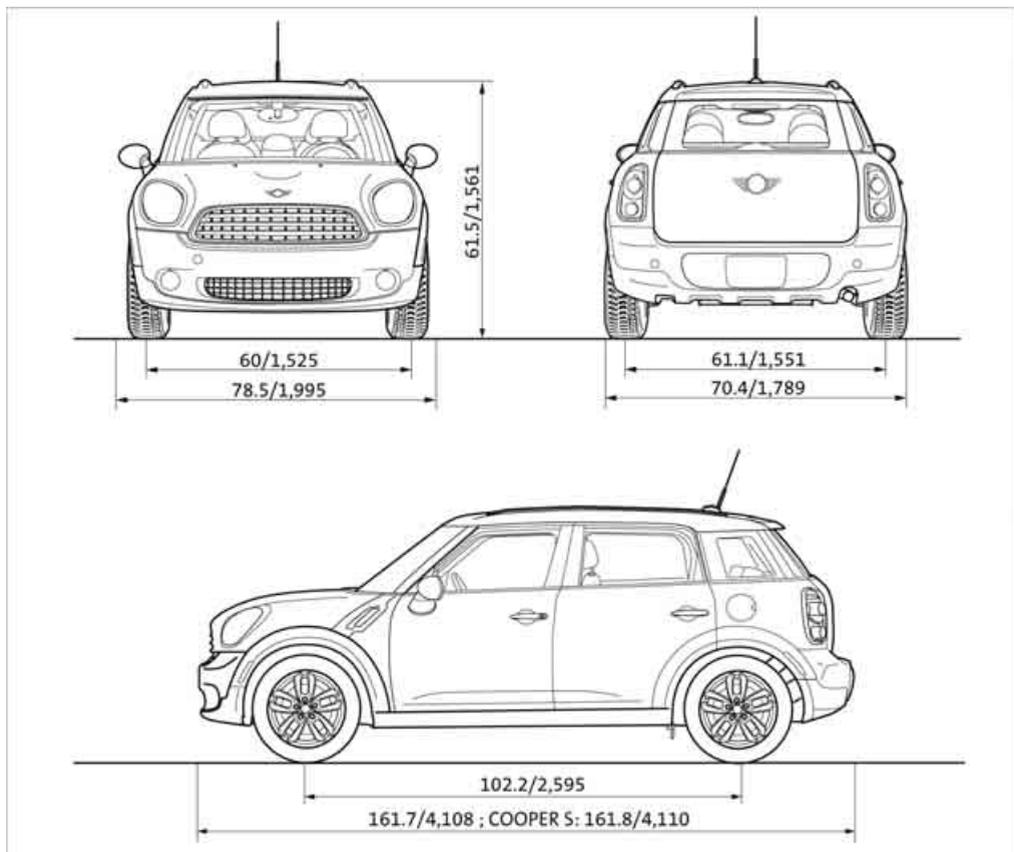
All dimensions in inches/mm. Minimum turning radius dia.: 38.1 ft/11.6 m.
