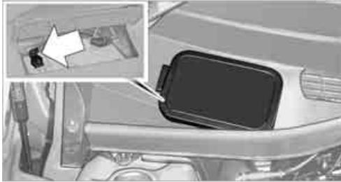
2. Release the tabs on the left and right sides of the positive terminal cover\*, arrows 1, and lift the cover to open, arrow 2.
