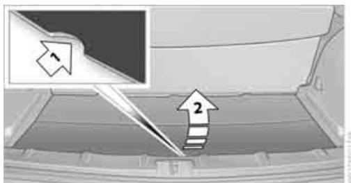
2. Lift up load floor behind and fold forwards, arrow 2.
