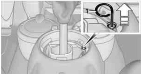
3. Insert extractor hook 1 into the loop on the passenger's side.
