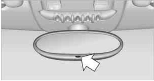
It is controlled by two photosensors:
