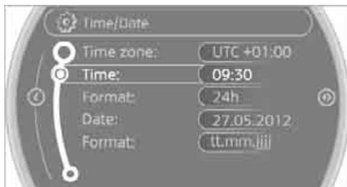
5. Turn the MINI joystick to set the hours and press the MINI joystick.
