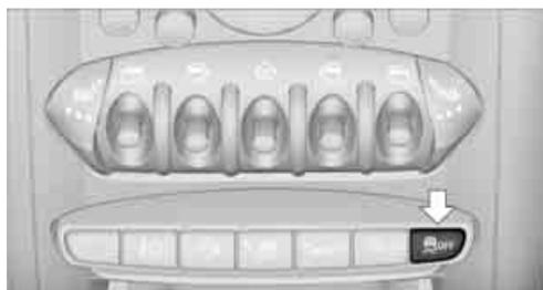
Press the button until the DSC OFF indicator light on the speedometer is on and DSC OFF is displayed on the tachometer. DSC is deactivated. Stabilizing and propulsion promoting actions are no longer executed.
