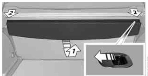
3. Release the locking mechanisms on the left and right sides, arrows 2.
