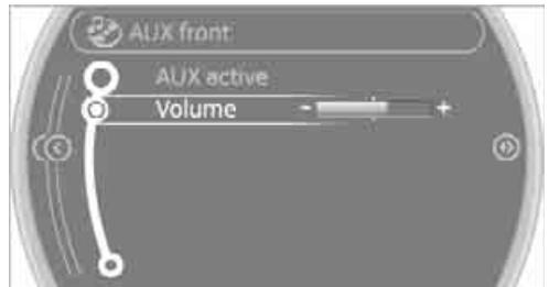
5. Turn MINI joystick until the desired volume is set and then press the MINI joystick.
