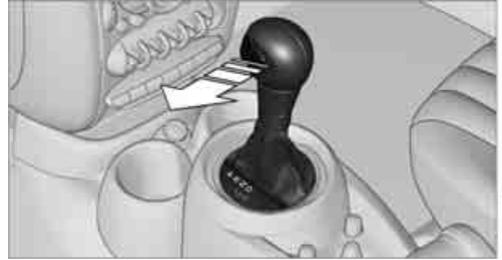
Move the selector lever from position D to the left into the M/S shifting slot: The Sport program is activated and DS is displayed. This position is recommended for a performance-oriented driving style.
