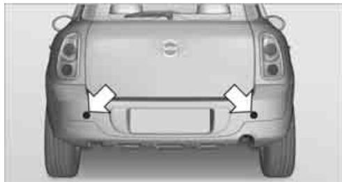
The mounting points are located under the covers in the bumper.
