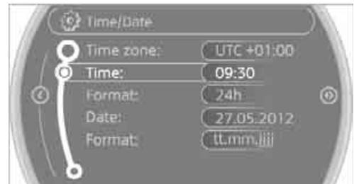
4. Turn the MINI joystick to set the hours and press the MINI joystick.
