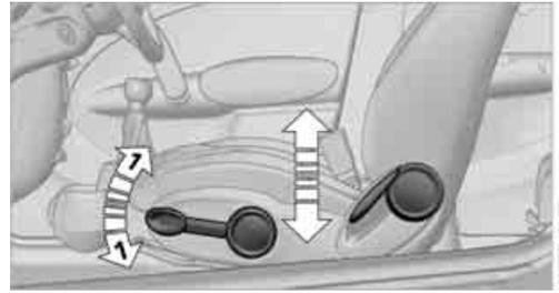
Pull up or push down the lever repeatedly, arrows 1, until the desired height is reached.
