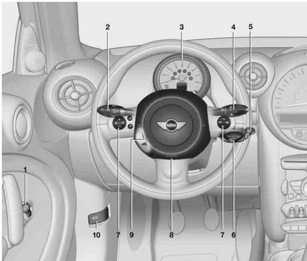
1 Adjusting the exterior mirrors, folding them in and out\* 36
