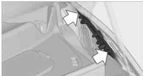
2. Squeeze clamping clip, arrows, and remove bulb holder.
