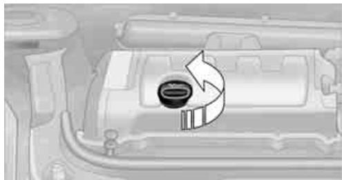
Do not add the maximum quantity of 1 US quart/1 liter of engine oil until the oil level has dropped to just above the lower mark on the dipstick, page 139.
