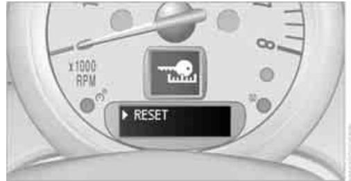
6. Press and hold the button until the display changes to the first setting. The settings are reset.
