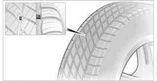
Wear indicators in the base of the tread groove are distributed around the tire's circumference; the letters TWI, for Tread Wear Indicator, on the tire's sidewalls identify tires that incorporate these wear indicators. If the tire tread has been driven down to the wear indicators, a tread depth of 0.063 in/1.6 mm has been reached.
