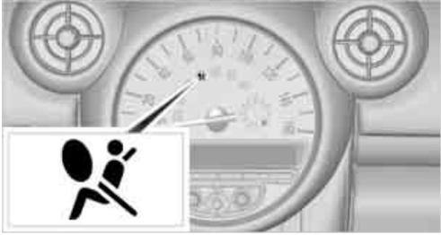
As of radio readiness, page 41, the warning lamp lights up briefly to indicate that the entire airbag system and the belt tensioners are operational.
