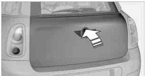
Press the top side of the MINI emblem, arrow, or Press the
