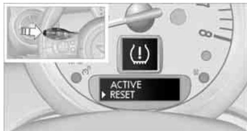
5. Press and hold the button until "RESETTING" is displayed.
