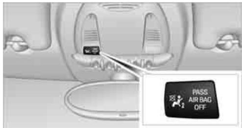
The indicator lamp for the front passenger airbags shows the functional status of the front passenger's front, side, and knee airbags in accordance with whether and how the front passenger seat is occupied. The indicator lamp shows whether the front passenger airbags are activated or deactivated.
