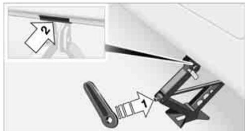
3. As you ratchet up the jack, place the jack head onto the lifting point on the body, arrow 2.
