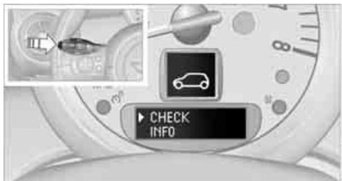
4. Hold the button down. If there are no Check Control messages, then "CHECK OK" is displayed. If a Check Control message has been stored, the corresponding message is displayed.
