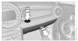
Press the button to open the cover. The light in the glove compartment comes on.
