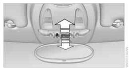
To switch the interior lamps on/off.
