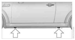
The vehicle jack is designed for changing wheels only. Do not attempt to raise another vehicle model with it or to raise any load of any kind. To do so could cause accidents and personal injury. 1. Place the jack at the jacking point closest to the wheel.
