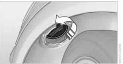
4. Screw out the bulb counterclockwise.
