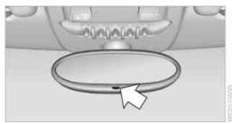
The automatic dimming feature of the interior rearview mirror\* is controlled by two photo cells in the mirror. One photo cell is in the mirror frame, arrow; the other is on the back of the mirror.
