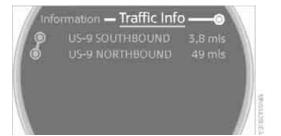
Traffic information on the planned route is shown first, sorted by distance from the vehicle's current position.
