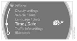
5. Turn the MINI joystick until "Time" is selected and press the MINI joystick.
