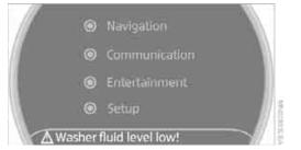
Text messages at the lower edge of the Control Display explain the meaning of the displayed indicator and warning lamps.
