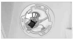
4. To insert the new bulb and replace the cover, proceed in reverse order.
