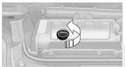
Do not add the maximum quantity of 1 US guart/1 liter of engine oil until the oil level has dropped to just above the lower mark on the dipstick, page 164.
