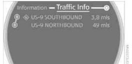
Traffic information on the planned route is shown first, sorted by distance from the vehicle's current position.
