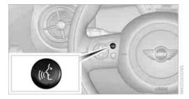
Inis symbol on the Control Display and an acoustic signal indicate that the voice command system is ready to receive spoken commands.
