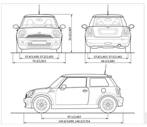
All dimensions given in inches/mm. Smallest turning circle diam.: 35 ft 10 in/10.7 m. Figures following the semicolons: Values that differ for the MINI Cooper S.
