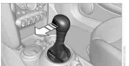
Move the selector lever from position D to the left into the M/S shifting slot: The Sport program is activated and DS is displayed.
