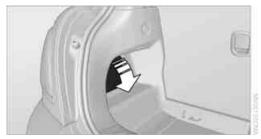
Screw out the desired bulb counterclockwise, arrows 1. Additional bulbs are located behind the sidewall of the cargo bay, arrow 2.
